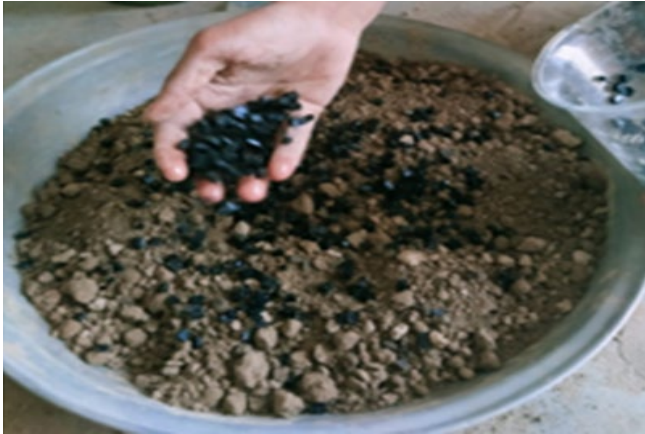
Fig. 3.1 Mixing tire rubber chips in soil
